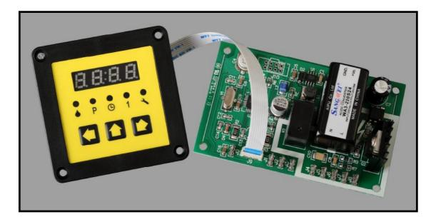
Universal Control Unit UC-2A is new type controller that designed for centralized lubrication system's control for chain lubrication like conveyor belt and escalator etc.
